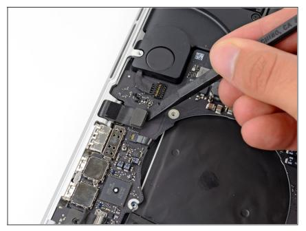
Use the flat end of a spudger to pry the headphone jack connector up from its socket on the logic board.
